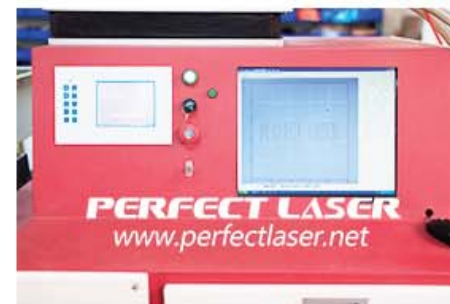
LCD Control Panel For Laser Power Supply
